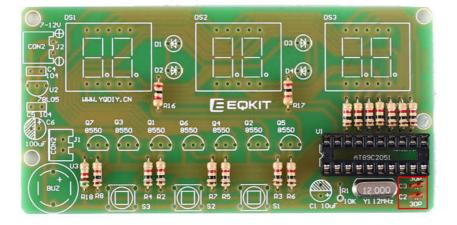
Step 7:Install 4pcs 3mm Red LED at D1~D4.Pay attention to the installation direction and the shorter pin is negative pins.
